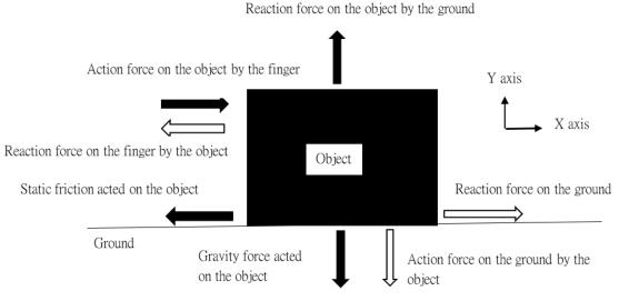
Figure 1: the object is in contact and relatively stationary with the ground
