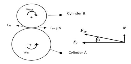
Figure 3. two contacted rotating cylinders
