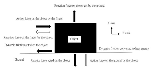
Figure 2. the object is in contact and moves relatives to the ground
