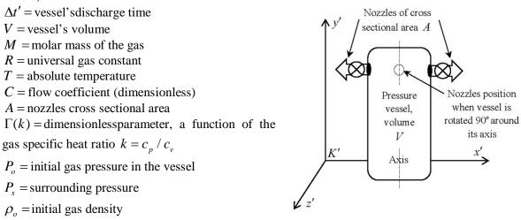
FIG. 1. Experimental arrangement
